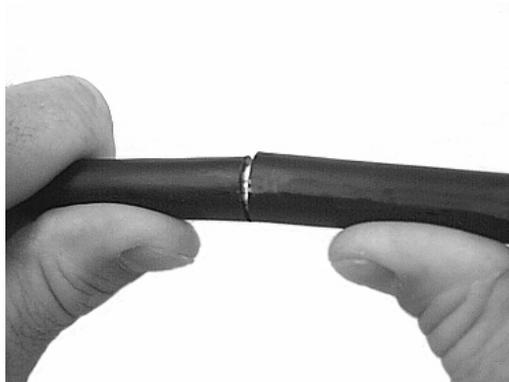
**Figure 11 – Flex the cable to separate the inner cable jacket.**
