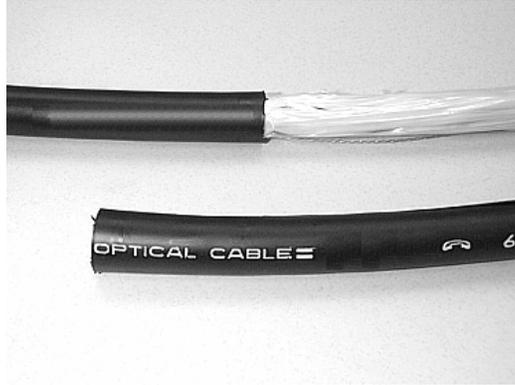
**Figure 24 – Remove the 5-inch section of cable jacket.**
