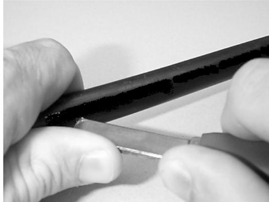
**Figure 4 - Make a longitudinal cut at the end of the cable.**
