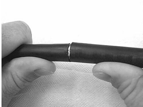
**Figure 22 – Separate the cable jacket.**
