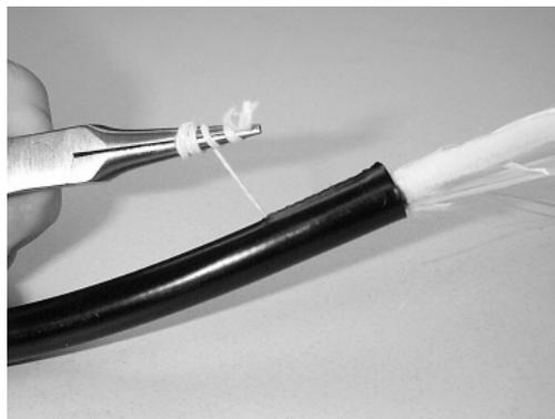
**Figure 14 - Pull the ripcord through the inner jacket.**
