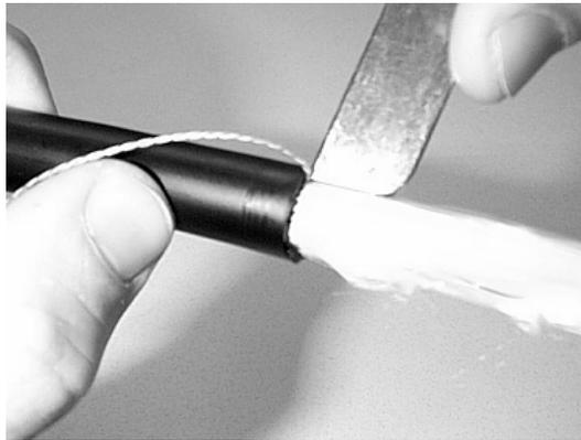
**Figure 25 – Cut a starting slit adjacent to the ripcord.**
