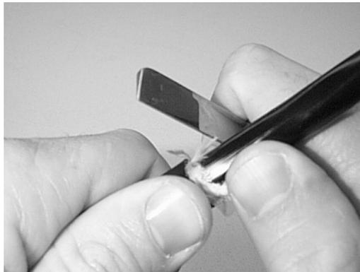
**Figure 10 – Ring cut the inner cable jacket.**
